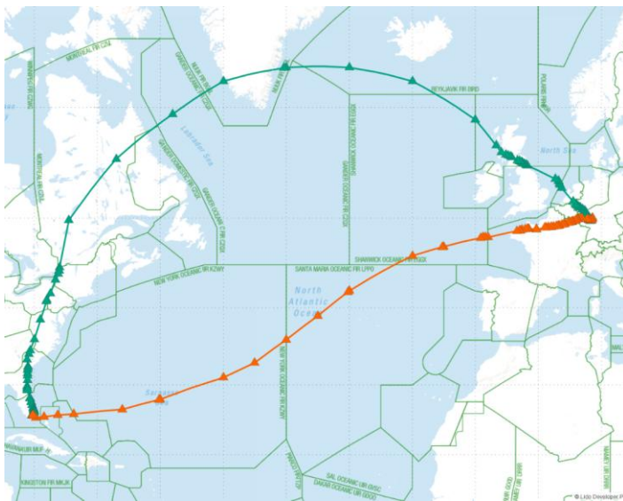
Figure 5: Optimized routes with non-CO 2 effects (green) and without non-CO 2 effects (orange) within the airspace structure (triangles).
