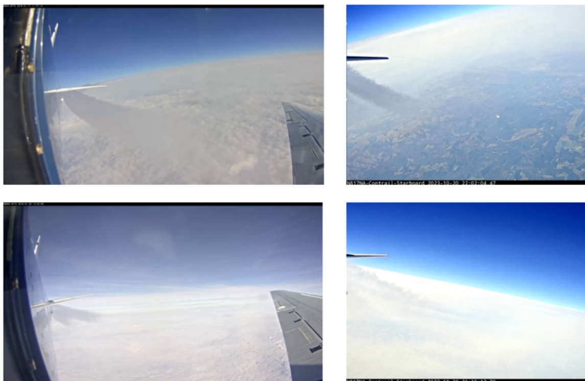
Figure 7. Comparison of the ND-MAX and ecoDemonstrator footage. (Top Left) ND-MAX campaign footage has tail obstruction in the view of the contrail, as well as a visible large portion of the aircraft fuselage and wing. (Top Right) ecoDemonstrator footage is not occupied by the aircraft body and the tail never covers the contrail stream. (Bottom Left) ND-MAX campaign footage is typically lower brightness and has a wider FOV, increasing the visible length of the contrail stream. (Bottom Right) ecoDemonstrator footage has high brightness and shorter view of the contrail.
