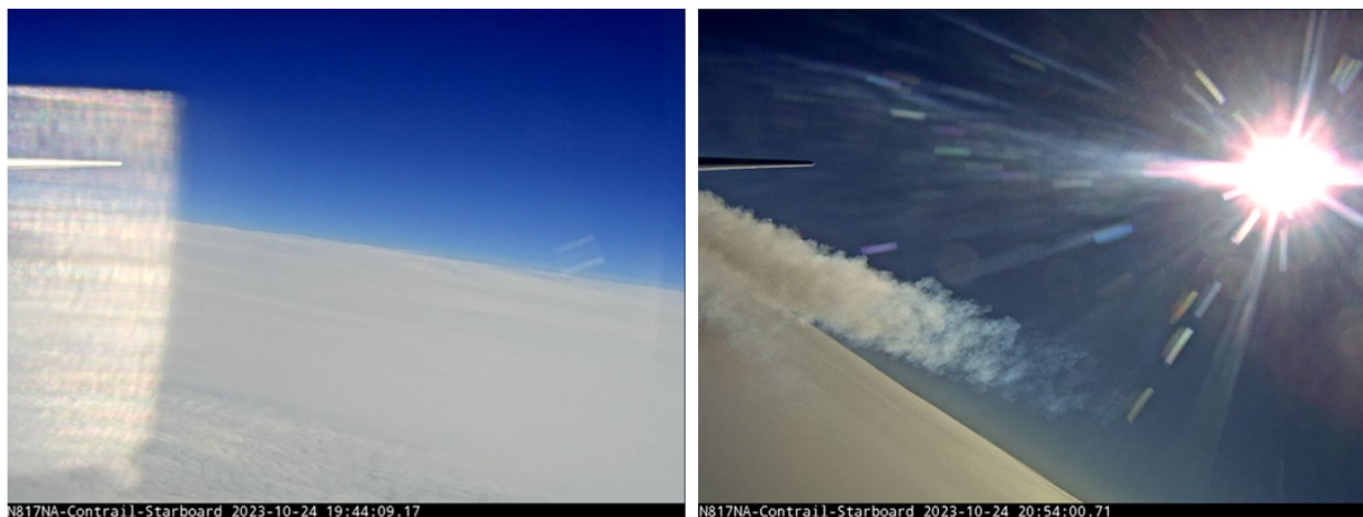
Figure 3. Camera view of two cases of sun glare. The left image shows an occluded contrail due to sun glare, while the right image retains visibility of the contrail despite the sun glare due to the positioning of the sun.
